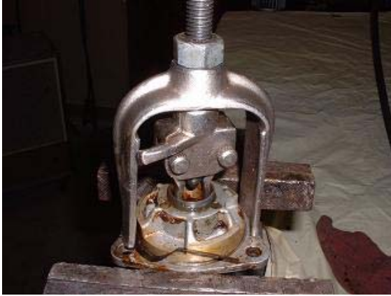
11. You will have to use a puller to remove the bushing from the cover. A pilot bearing puller works well here. Replace all the bushings .
