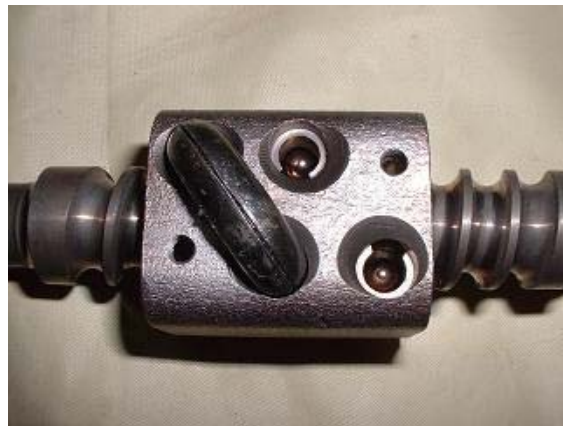
22. Install both ball guides. If they don't seem to want to go in make sure they are centered in the holes and tap gently with a hammer.
