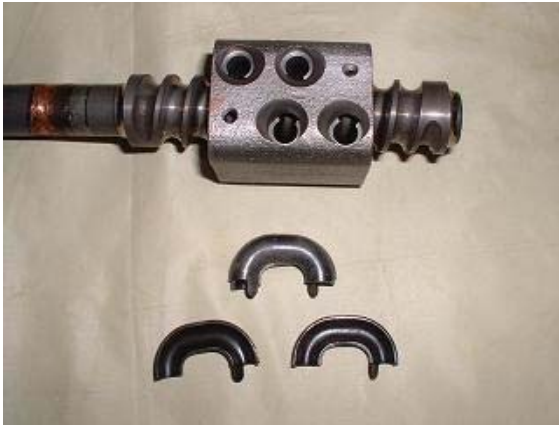
19. Notice the tabs on the end of the ball guides. If the worm nut is allowed to run all the way to the end (when assembled) it could bend these tabs.
