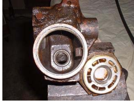
12. Clean out some of the grease then check the bearing races for pitting, scratches or discoloration. Replace if any problems are found.
