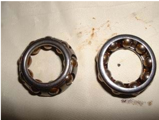
13. Check the bearings also. Check each ball carefully and replace if necessary. The balls can be replaced (as a set) but you'll still need the shells.
