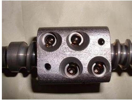
20. Insert the new worm nut on shaft. Now count out 36 balls in groups of 4 and insert one in each hole. Repeat until all 36 balls are inserted.
