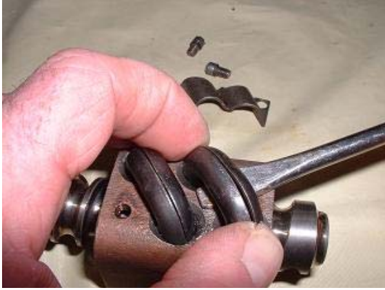
17. Start disassembly by removing the ball guides. Pry them straight up evenly with a screwdriver to prevent bending the tabs.
