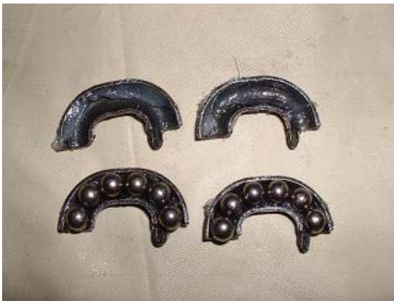
21. Smear some grease in all 4 of the guides then place 6 balls in each of 2 of the guides. Now place the guide halves together.
