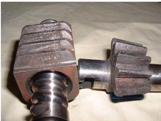
15. This is what you don't want to find. The gears are galled and must be replaced. This is usually caused by over tightening the adjusting screw.
