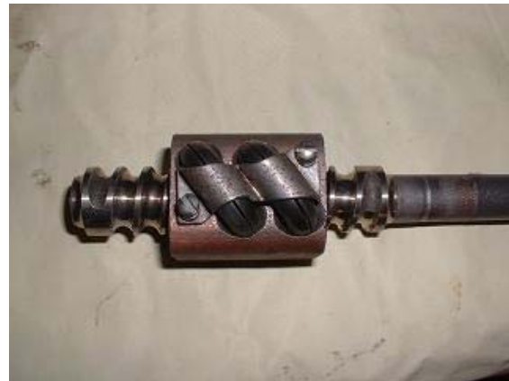
14. Do Not disassemble this unless absolutely necessary. If it turns smoothly end to end leave it alone. Also don't let spin to the end on its own.
