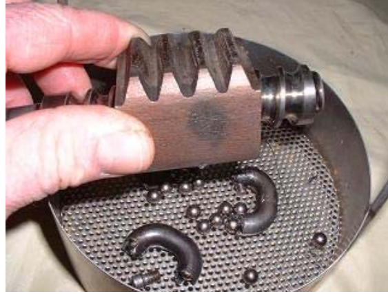
18. Shake, twist and turn all 48 balls out of the worm nut into a suitable container. Clean and inspect all components.
