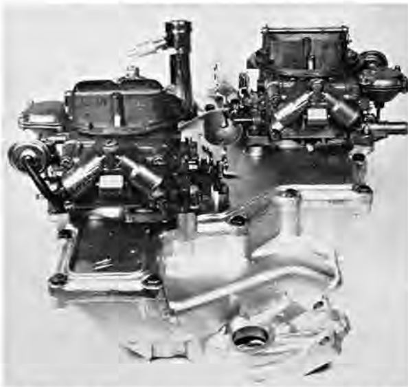
Here's 25 horsepower worth of "spankin' new" Chevy manifold from Chevy. Parts number is included in the story. Lid removal facilitates attachment of manifold to engine. Short-ram principle is well liked by the little Stovebolt.
